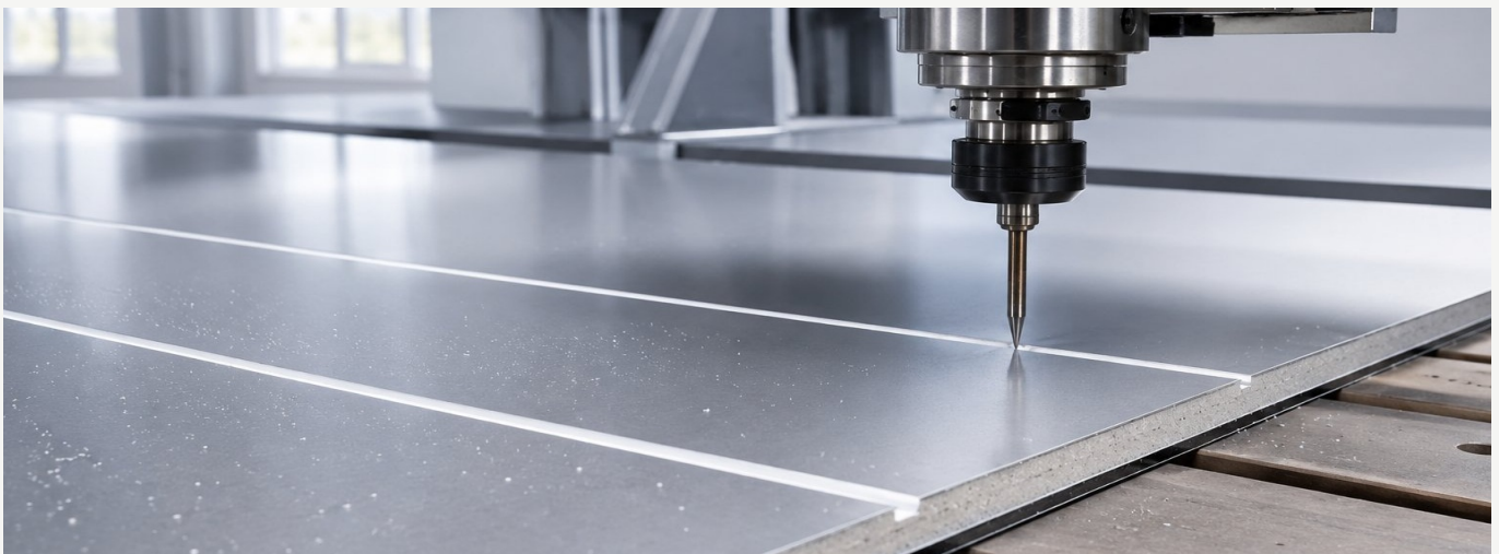
CNC ROUTER PERFORMING PRECISION V-GROOVE ROUTING ON ACP FR CORE B1 PANEL.
